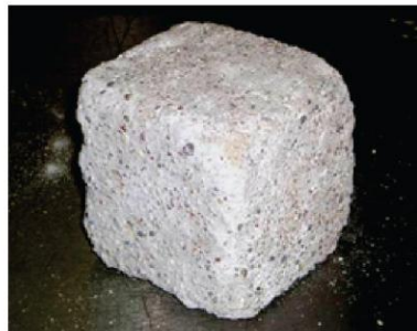
100% OPC concrete after exposure to silage acid showing significant deterioration
