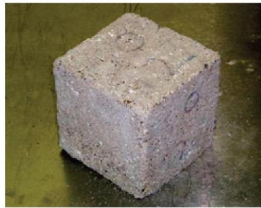
50% GGBS concrete after exposure to silage acid showing little deterioration
